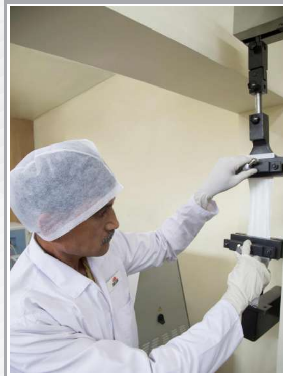
Tensile Testing Machine for all inputs used in FIBC with load bearing capacity upto 5000 N (500Kg).
