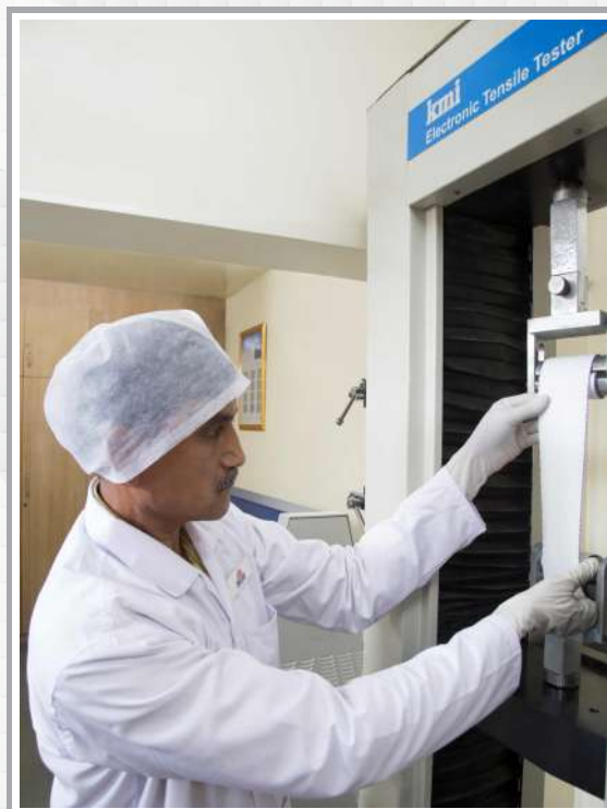
Tensile Testing Machine for all inputs used in FIBC with load bearing capacity upto 5000 N (500Kg).
